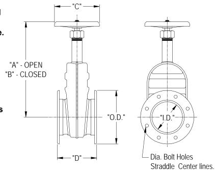
See section 18 Page 4A for parts list. Flanges are Drilled to TTMA Recommendations.
